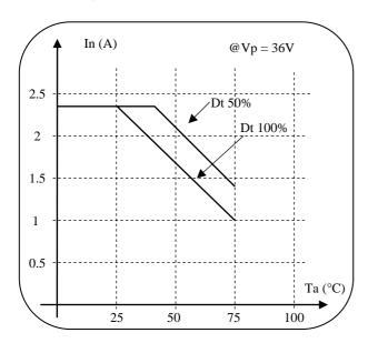
It is important to take note that if the working cycle is at 50%, the reachable current limit is much higher compared to a motor driver continuously working.
