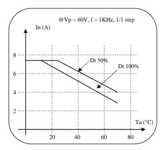
It is important to take note that if the working cycle is at 50%, the reachable current limit is much higher compared to a motor driver continuously working.
