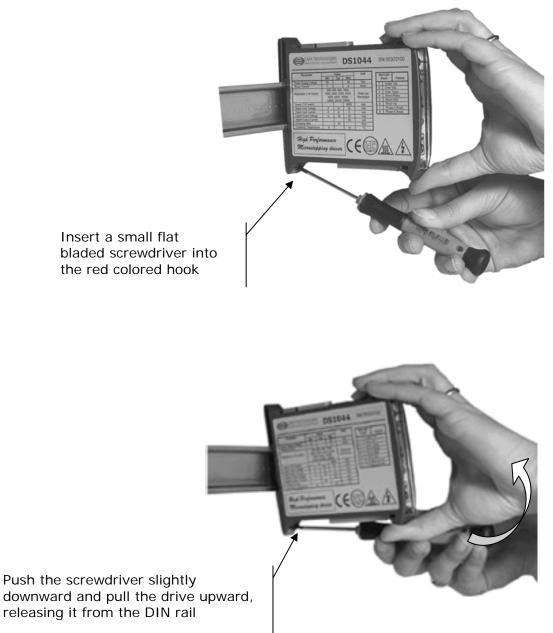
downward and pull the drive upward, releasing it from the DIN rail
