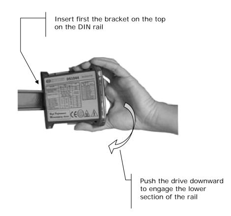
To remove the drive from the DIN rail insert a small flat bladed screwdriver into the red colored hook on the bottom, on the back of the drive. Push the hook downward and pull the drive upward slightly rotating it, releasing it from the DIN rail as shown in the picture.
