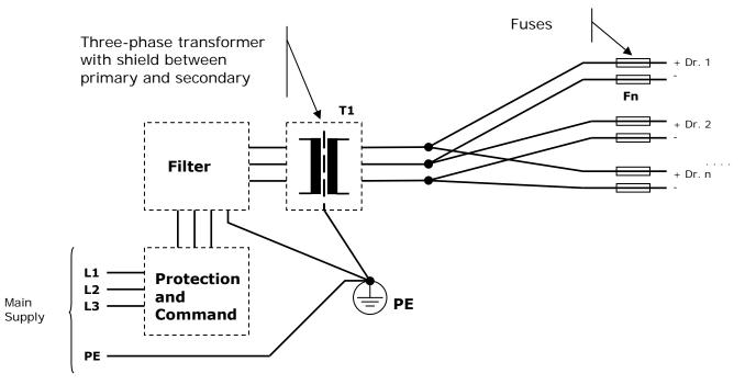
The above scheme includes a three-phase transformer (note the distribution of the drives on the three phases). If necessary it is also possible to use a mono-phase transformer.
