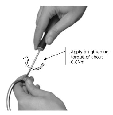
All terminals can tighten correctly cables with section between  $0.1 \text{mm}^2$  and  $2.5 \text{mm}^2$  (24...14 AWG).
