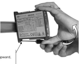
Push the screwdriver slightly downward and pull the drive upward, releasing it from the DIN rail
