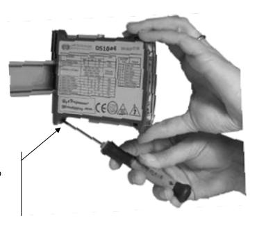
Insert a small flat bladed screwdriver into the red colored hook
