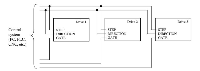
In this case the control system sends a step and direction signal to all the drives contemporaneously, while the GATE signal is activate from time to time on the only drive the control system wants to move. The drives with the GATE signal not activate ignore the pulses and maintain the motor firm.
