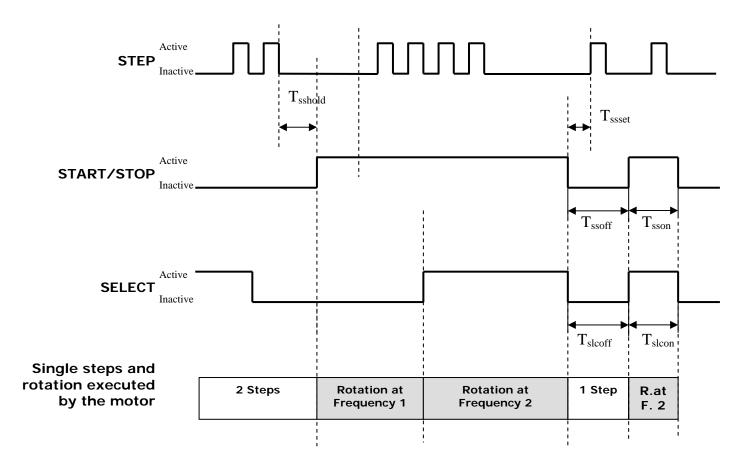
To grant a correct execution of the given commands it is necessary to respect some time relations among the signals. In the following table are detailed the limits to be observed.
