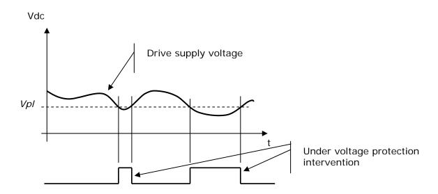
If the supply voltage is very near to the drive functioning limit and sporadically the under voltage alarm intervenes, it is possible, in some cases, to solve the problem reducing the distance between the power supply and the drive, increasing the cables section or placing an electrolytic capacitor near the drive itself (valid only the DC models).
