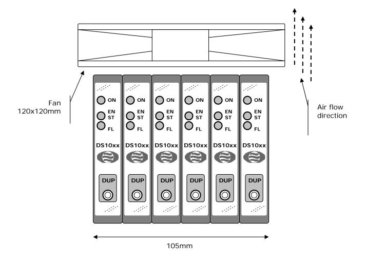
In case of a reduced fan size, it must be set in a rear position and at about 30mm high from the drive. A nearer or more distant position could reduce its effectiveness.
