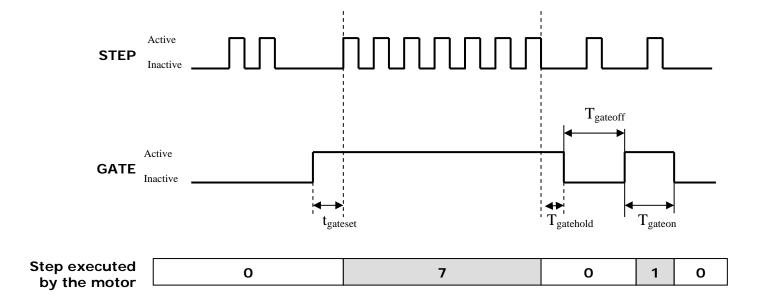
To grant a correct execution of the given commands it is necessary to respect some time relations amongst the signals. In the following table are detailed the limits to be observed.
